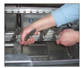
Remove the pawl bar by grapsing firmly and lifting up.
